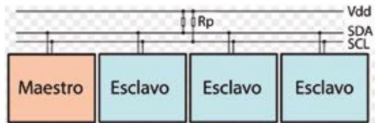
Figura 1. PMBus de MW
