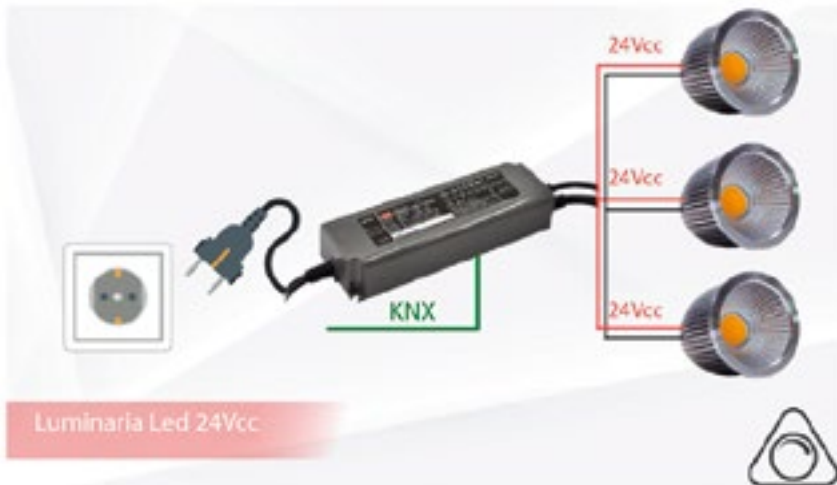
Figura 6. LED driver KNX con luminarias LED de 24Vcc.
