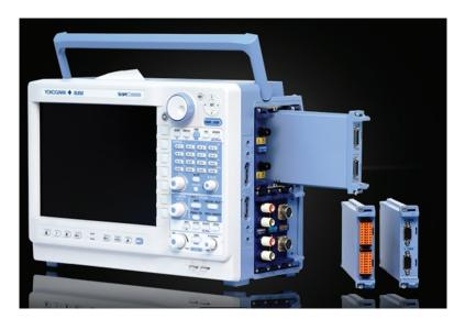
USB ports, an Ethernet port, an e-SATA port, a video port, a GPIB port, and a SD-card slot populate the unit's left side panel. On the right side, the DL850 has room for eight input modules.
