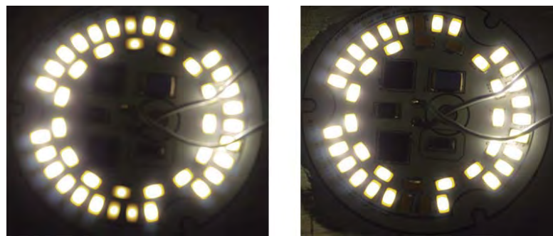
Figure 2d. LED module dimmed to 6 W: the luminous flux modulation is approx. 9 ms. Six LEDs are already less bright.
