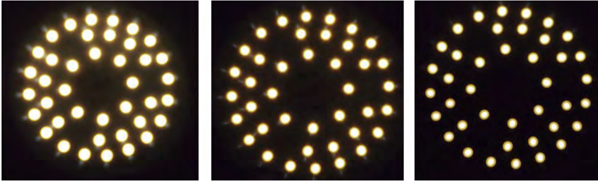
Figure 2. The EL01 LED modules can easily be dimmed without changing the luminous flux modulation:
