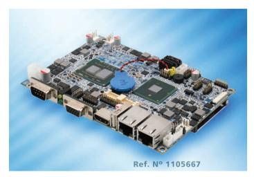
Utilizing the low voltage Intel® Core i7-620LE or the ultra-low voltage Intel® Core i7-620UE processor, the ECM-QM57 is adopted with the latest Intel® QM57 Express chipset.
