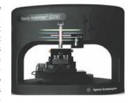
flexible and user-friendly instrument for nanoscale mechanical testing, the G200 utilizes electromagnetic actuation to achieve unparalleled dynamic range in force and displacement. The G200 enables measurement of Young's modulus and hardness in compliance with ISO 14577, as well as measurement of deformation over six orders of magnitude – from nanometers to millimeters.
