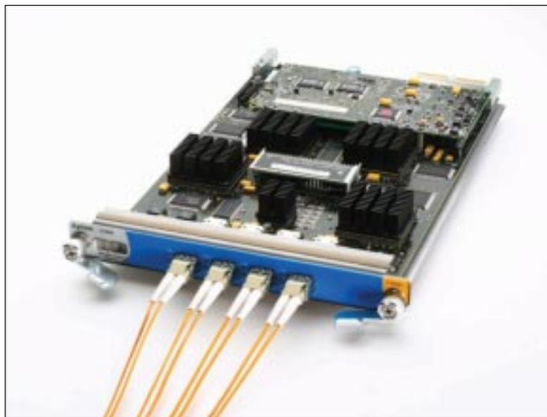
Figura 1. Tester SUN con cuatro ports Fibre Channel (2Gbs & 4Gbs)
