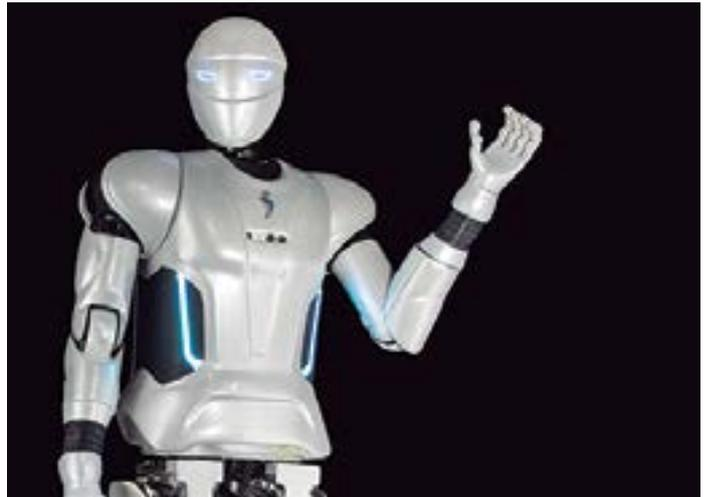
*SURENA III is a humanoid robot capable of climbing stairs, recognizing speech, communicating and navigating*
