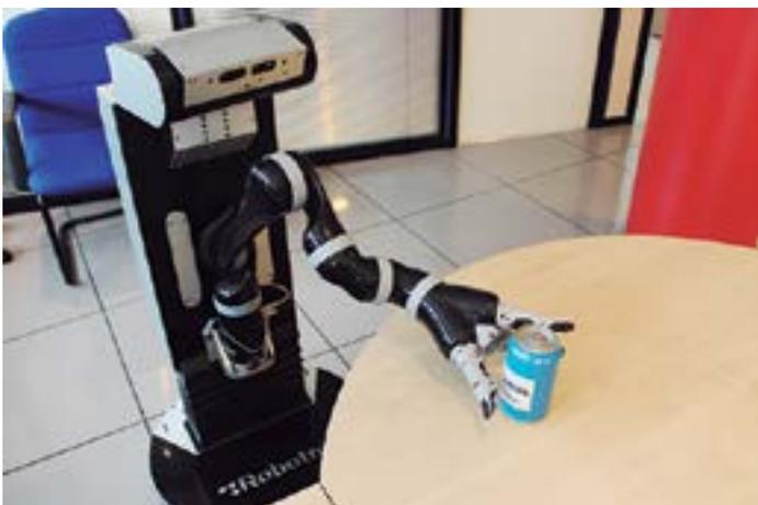
*RB-1 is a new autonomous and configurable robot developed for remote handling and Ambient Assisted Living. Featuring 6 DOF, RB-1 can incorporate a two or three fingered gripper, enabling users to interact with their environment in total safety.*
