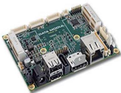
**eDM-pITX-BT – Industrial Pico-ITX SBC based on latest Intel® Atom™ E3815/ Celeron J1900processors**
