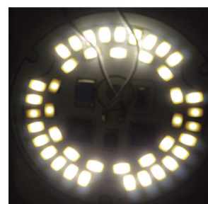
Figure 5. Some solutions in the market switch off individual LEDs during dimming - top: 4 W, bottom: 6 W.
