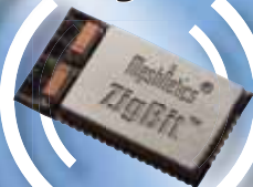
ZigBit Dual Chip 24x13,5mm
