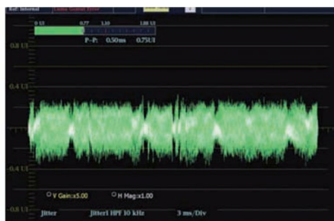
With the 10kHz filter applied to the signal the jitter read indicates a value of 0.75UI. A more horizontal trace of the jitter waveform is observed.
