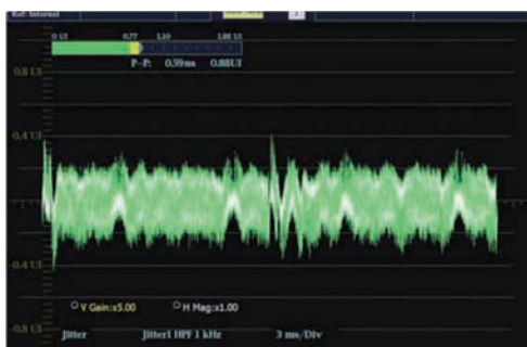
The jitter readout with the 1kHz selection now reads 0.88UI showing a slight increase in the jitter present within the signal and one can observe a differentiation occurring at field rate with this filter applied. This indicates a component of jitter present on the band-pass edge.
