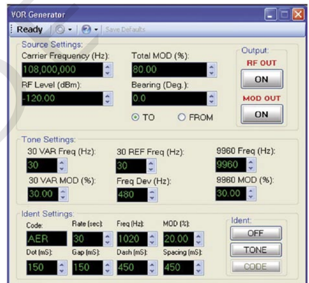
Figura 3. VOR Generator, pantalla principal
